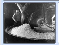
The woodchip is soaked in water and turned into **pulp** in a large machine. Bleach is added to the water to clean the paper and turn it white.
