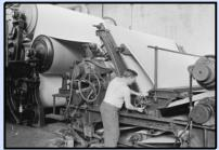
The pulp is then transferred to the **paper-making machine**. In this machine it is pressed, dried and cut. All the paper comes out of the machine the same colour, size and thickness.
